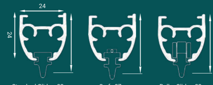
Standard Glider - 33mm Surf - 37mm Roller Glider - 33mm Surf Roller Glider - 38mm
